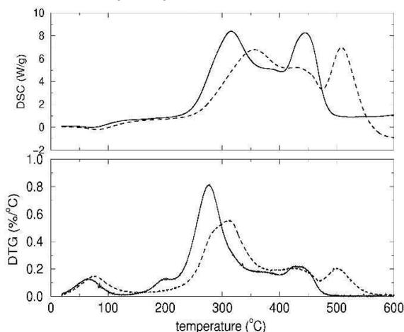
Fig. 3. DSC curves (top) and DTG curves (bottom) for untreated sample (continuous line) and sample with boric acid (dashed line).
