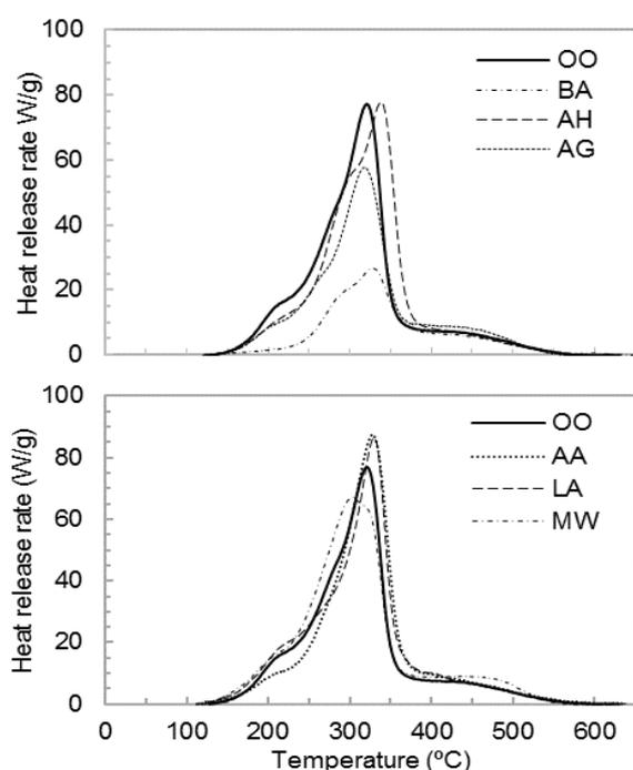
Fig. 1. Heat release rate as a function of temperature for specimens incorporating boric acid, aluminium hydroxide and sodium alginate (top) and montan wax, acetic acid and lactic acid (bottom). Results are compared with plain boards (OO).
