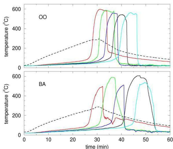
Fig. 5. Temperature evolutions for thermocouples located each 3 cm along the sample for untreated (top) and boric acid fire retarded (bottom).
