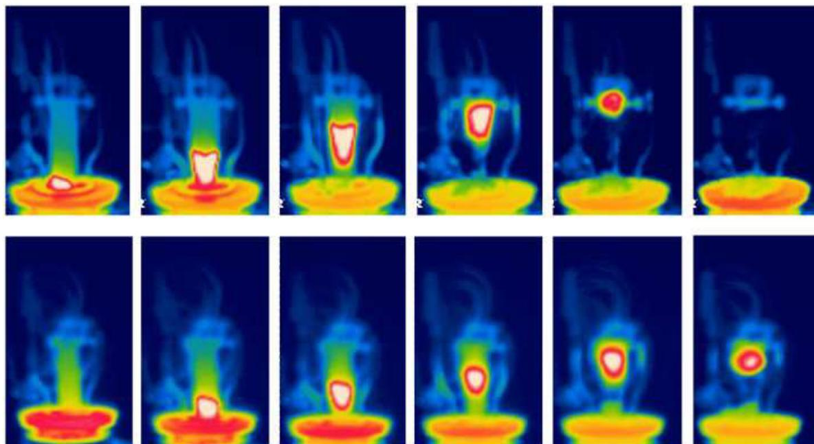
Fig. 4. Infrared images for untreated (top) and boric acid fire retarded (bottom) at times  $t=30, 35, 40, 45, 50$  and  $55$  min
