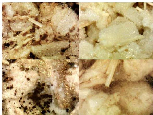
Fig. 7 Images of the mould affection of four different specimens.
