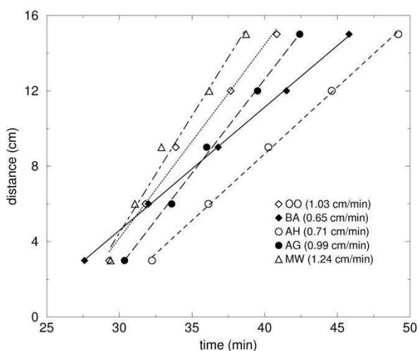
Fig. 6 Thermocouple position versus time at which temperature reaches 250°C for the different samples analysed. Smouldering propagation velocities (shown in the inset of the figure) are calculated as the slope of the obtained lines.
