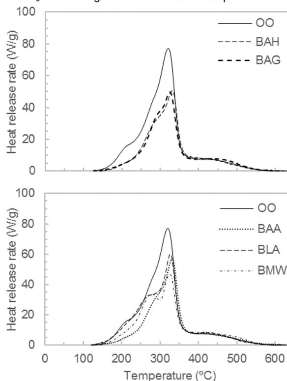
Fig. 2. Heat release rate as a function of temperature for specimens incorporating boric acid and one of the other additives. Results are compared with boards containing only boric acid (BA).
