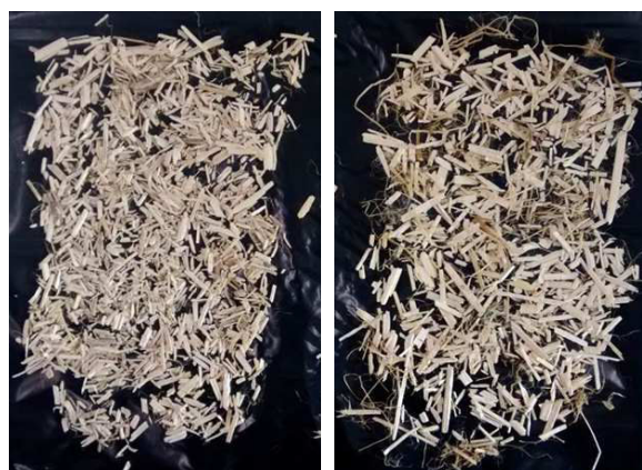
Shiv A Shiv B Fig. 1: Two types of hemp shiv in bulk
