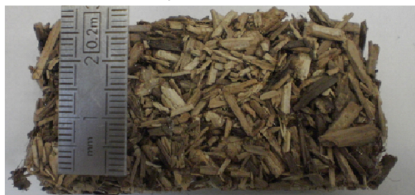
Fig. 1: PLA Hemp Composite specimen.
