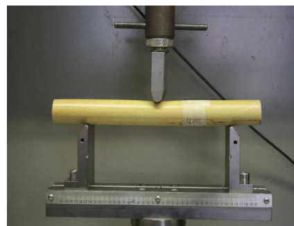
Fig. 2: Three point bending test.
