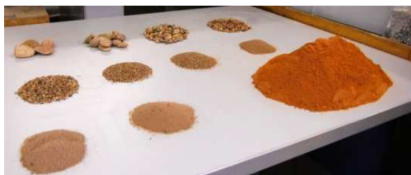
Fig. 1: Different particle size fractions of the clayey sand used for the plasters.
