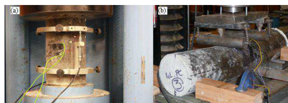
Fig. 2: Axial compression (a) and four point bending (b) test.
