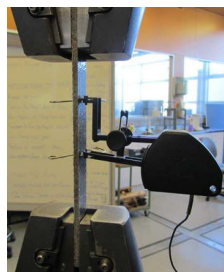
Fig. 3: Tensile test of flat-coupon FFRP laminate.
