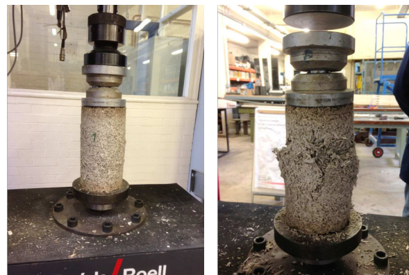
Fig 5: Mode of failure of cylinder 11x22 cm.
