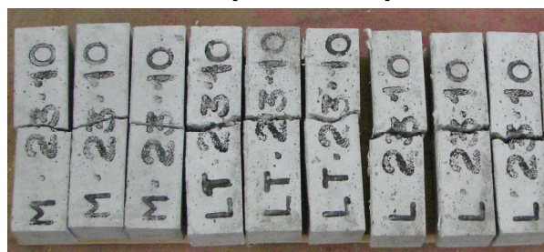
Fig. 4: The specimens tested in three point bending.
