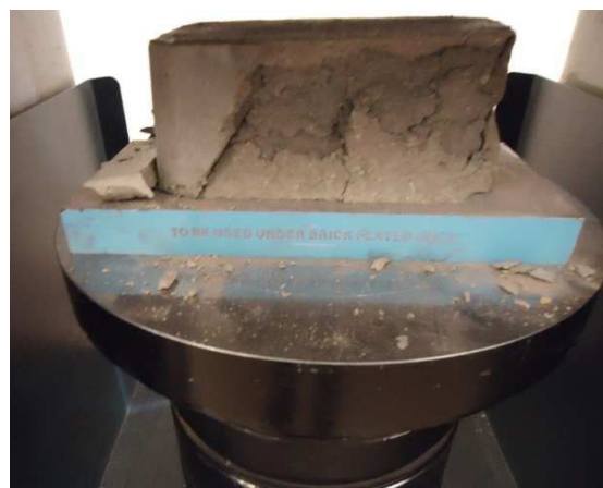
Fig. 10: Failure pattern of SCEB [Egenti 2014]
