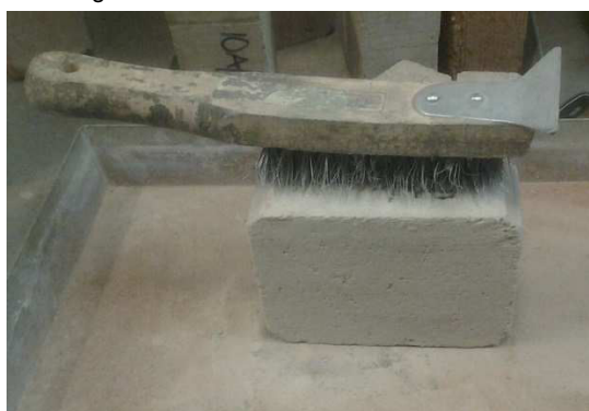
Fig. 8: Wire brush test of surface abrasion
