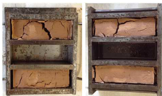
Fig.5: Specimens of earth/starch mixes (with starch J on the left and starch K on the right).
