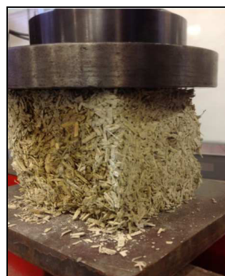
Fig. 1: Typical failure of hemp concrete under axial compressive.
