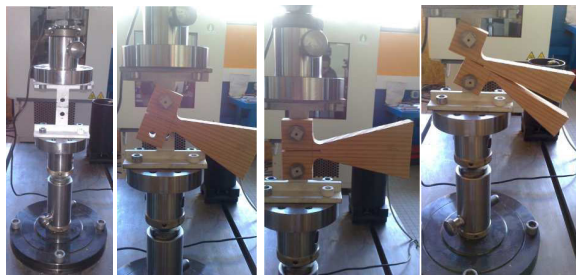
Fig. 1: Experimental device (Douglas Fir).
