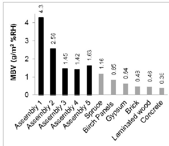
Fig. 6 : Comparison of moisture buffer value of the assemblies of the present test with that of other building materials determined by NORDTEST.
