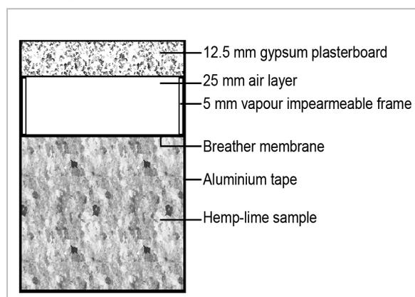
Fig. 2 : Vertical cross section of assembly 4
