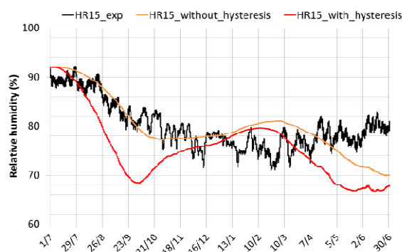
Fig. 19: Evolution of RH at depth 15cm: comparison between Matlab models with and without hysteresis
