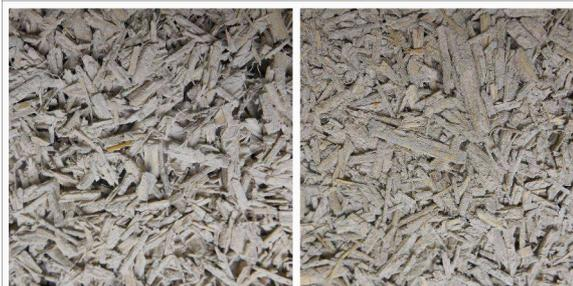
Fig. 6: Surface of low density ( $210 \text{ kg/m}^3$ , upper) and high density ( $333 \text{ kg/m}^3$ , lower) samples showing spaces between hemp particles
