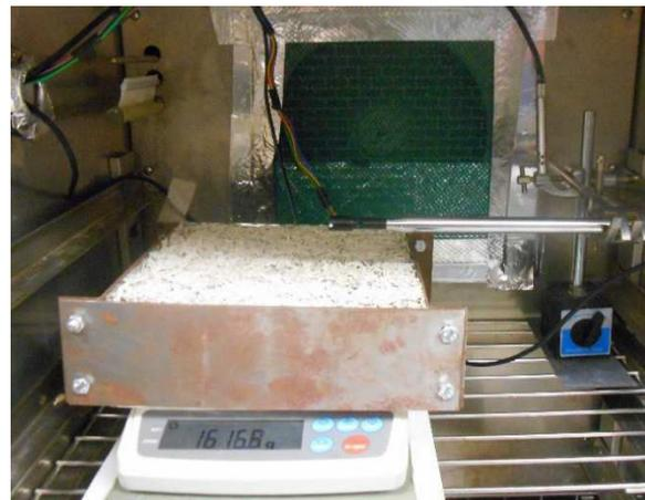
Fig 1: Climate chamber with sample and anemometer.
