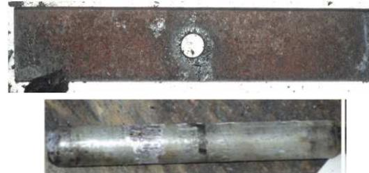
Fig. 5 : Heating of dowel and metal plate.
