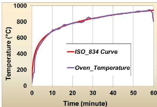
Fig. 4 : ISO 834 temperature-time evolution
