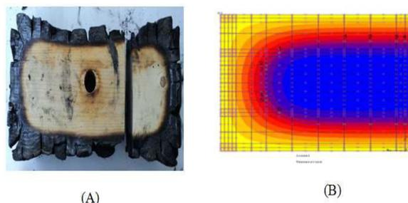
Fig. 10 : experimental and numerical carbonization.
