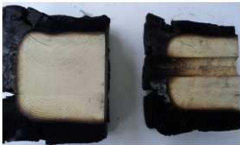
Fig. 3 : Carbonization of timber members.
