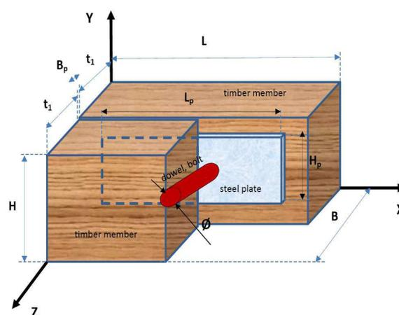
Fig. 2 : Geometrical dimensions.
