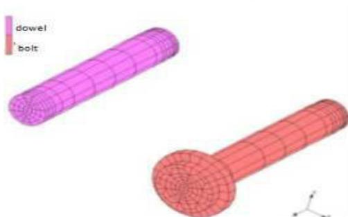
Fig. 9 : FEM modeling of bolt and dowel.
