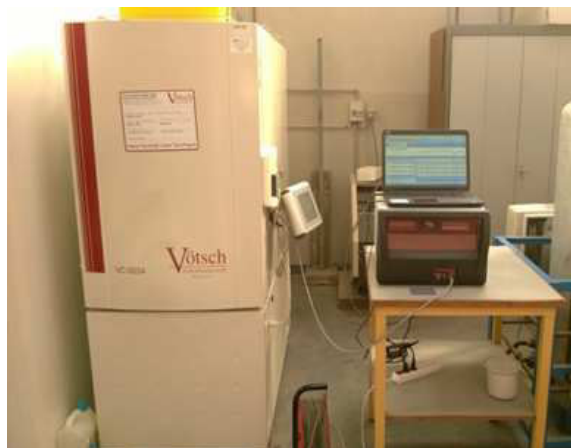
Fig. 1 : Measurement of thermal characteristics in climatic chamber
