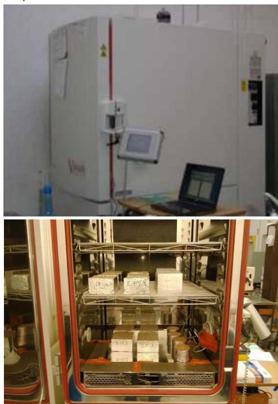
Fig. 2: Measurement of Moisture Buffer Value: experimental device and specimens
