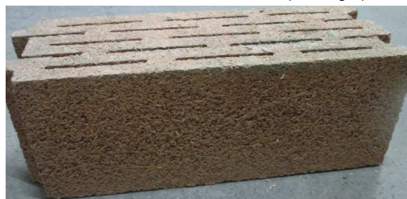
Fig. 1: Hemp shives-based precast block (SEAC).
