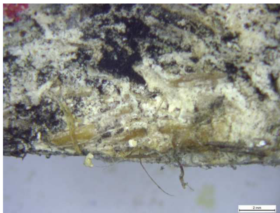
Fig. 3: Example of fungi growth on the surface of hemp-lime mortars subjected to intense wet-dry cycles.
