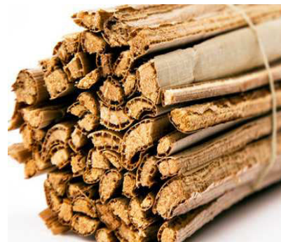
Fig. 4: Typha bars after longitudinal cut, as basis for the production of Typhaboard.
