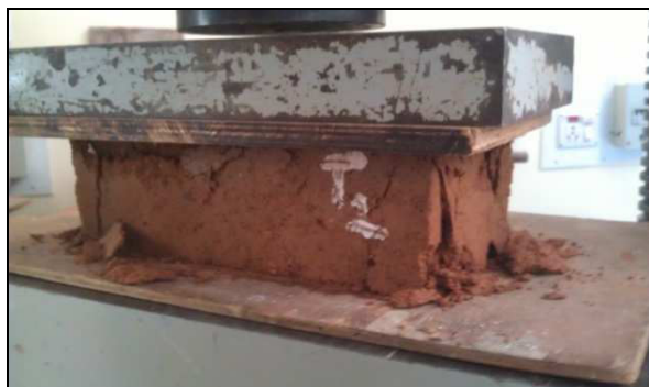
Plate 2: View showing the testing of CSEBs for its Wet Compressive Strength
