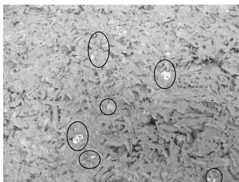
Fig. 3: Mould on blocks (enclosed areas).
