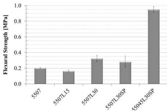
Fig. 8: Flexural strengths of prisms.
