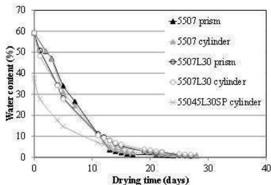
Fig. 4: Drying curves of laboratory samples.
