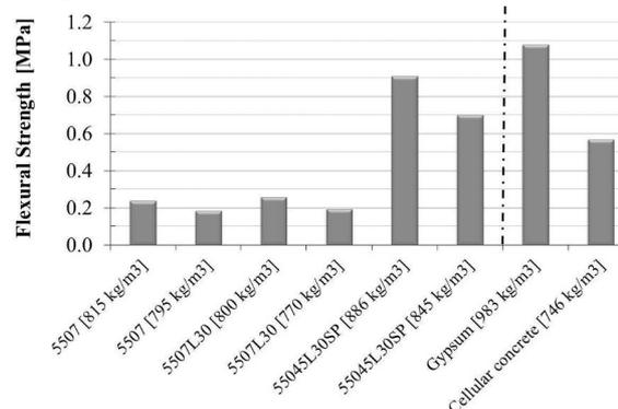
Fig. 9: Flexural strengths of blocks.
