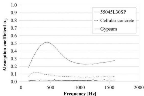
Fig. 11: Acoustic absorption coefficient of blocks.
