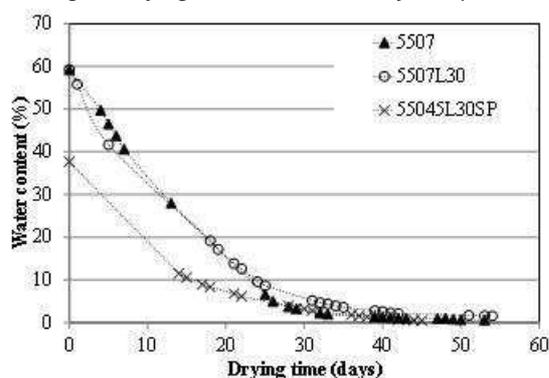
Fig. 5: Drying curves of blocks.
