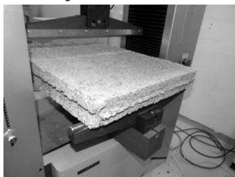
Fig. 2: Block made with quarry fines and hemp straw (mix 55045L30SP) - Three point bending test.
