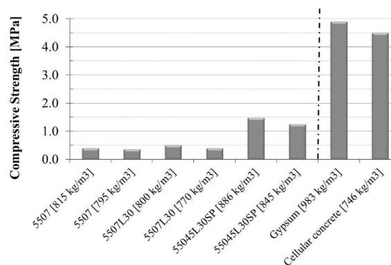
Fig. 10: Compressive strengths of blocks.
