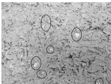
Fig. 3: Mould on blocks (enclosed areas).
