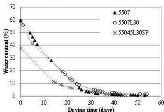
Fig. 5: Drying curves of blocks.
