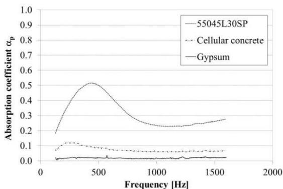
Fig. 11: Acoustic absorption coefficient of blocks.
