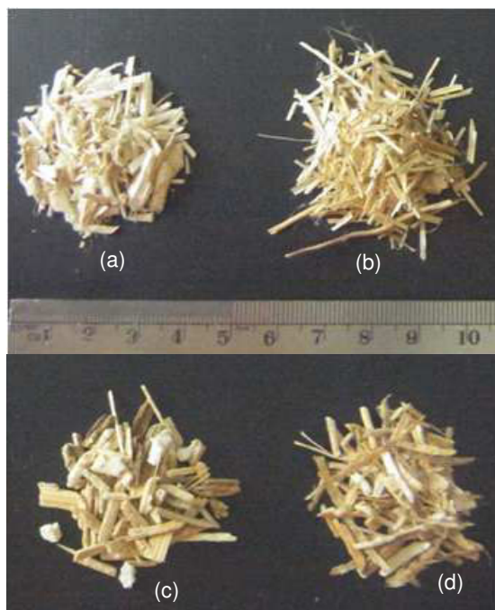
Fig. 1 : Sample of hemp shives (a), flax shives (b), sunflower bark (c) and rape straw (d).
