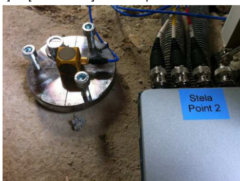
Fig. 10 : Vibrational measurements by triaxial accelerometers.
