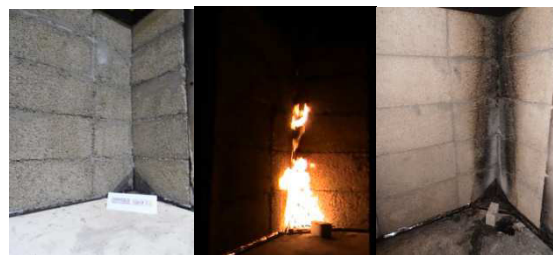
Fig.2: Demonstration of fire reaction test on hempcrete blocks at CREPIM
