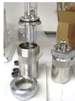
Fig. 3: Calorimetric bomb for the Gross Heating Value GHV determination – CREPIM device
