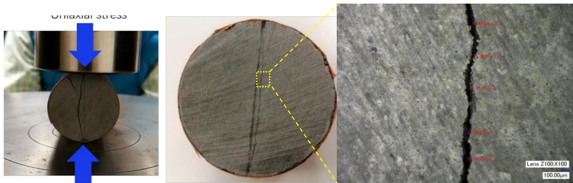
**FIGURE 2.** Creation of a diametral macro-crack in a cylindrical COx claystone sample by using a Brazilian splitting test
