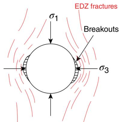
**FIGURE 1.** Diagram of the Excavation Damaged Zone (EDZ) around a tunnel, from (Bossart et al., 2019)
