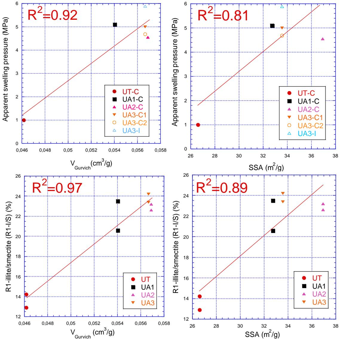
**FIGURE 6.** Correlation of nitrogen adsorption data with apparent swelling pressure  $P_{app}$ : (a)  $P_{app}$  vs.  $V_{Gurvich}$  (b)  $P_{app}$  vs.  $SSA$  (c) R1-I/S vs.  $V_{Gurvich}$  (d) R1-I/S vs.  $SSA$
