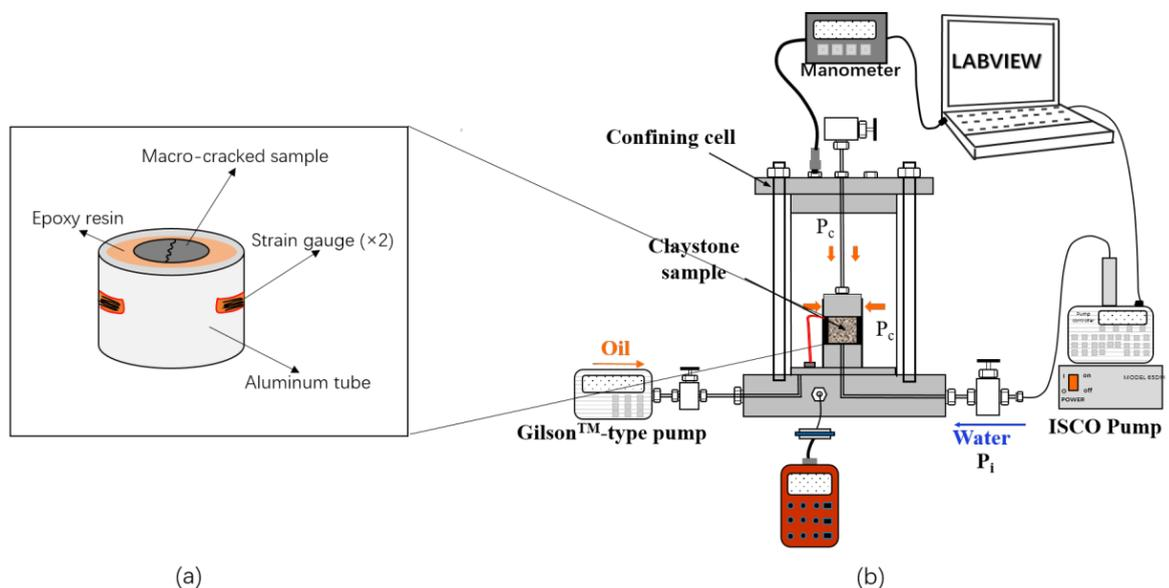
**FIGURE 3.** Sketch of the experimental set-up: (a) a mock-up formed by the sample surrounded by an aluminum-epoxy tube avoids that external stress are applied to the sample; (b) the hydrostatic triaxial cell used for the swelling and self-sealing experiments.
