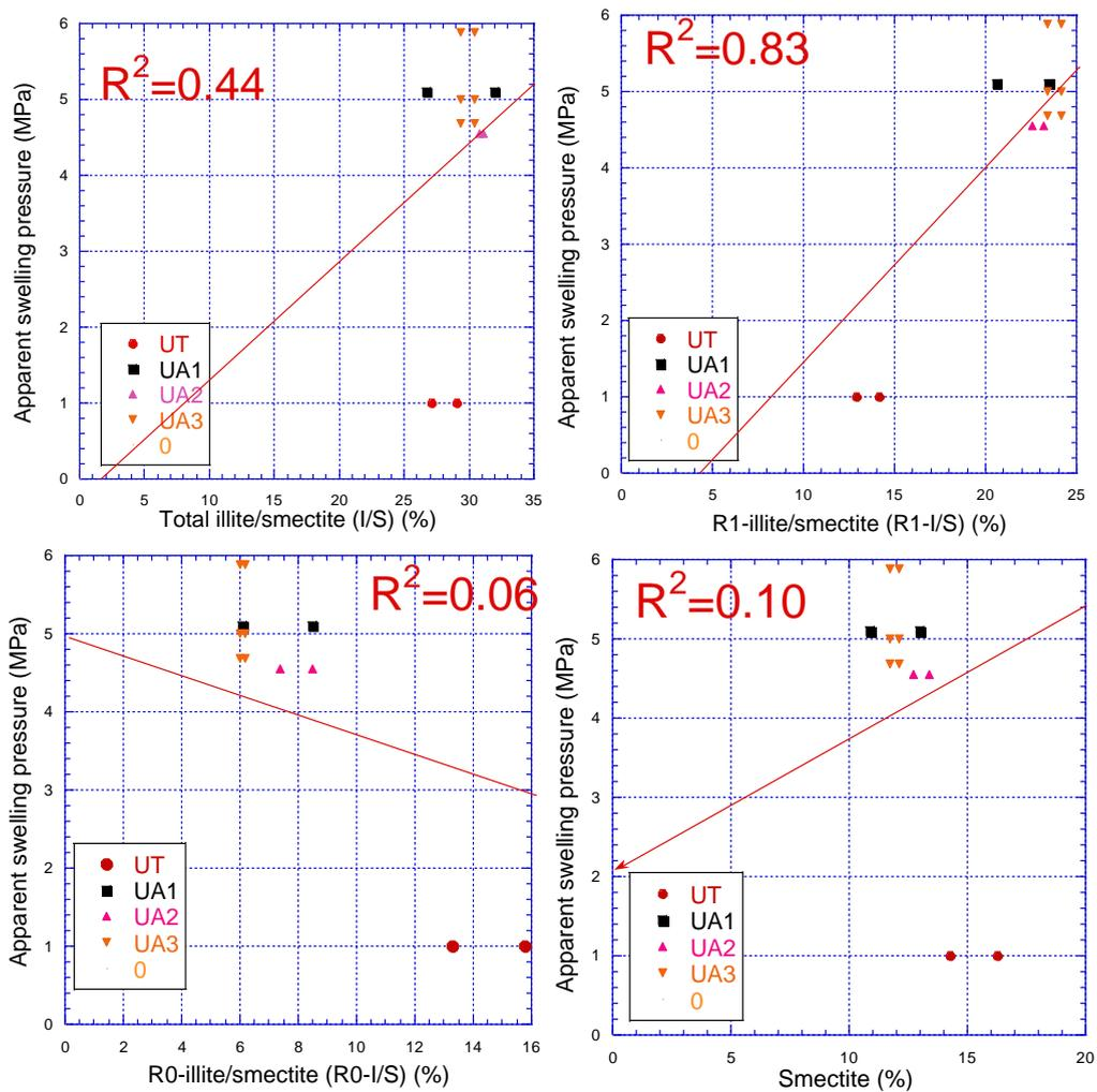
**FIGURE 5.** Apparent swelling pressure  $P_{app}$  as a function of specific clay mineral content
