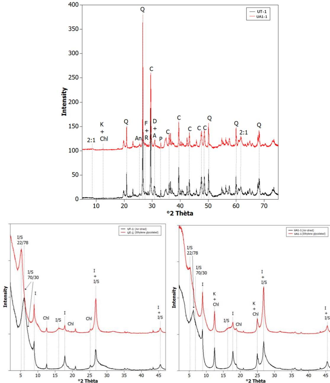
FIGURE 4. XRD spectrum examples of the bulk powder and oriented clay fractions (UT-1 and UA1-1)
