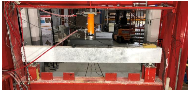
FIGURE 1 Bending test set-up
