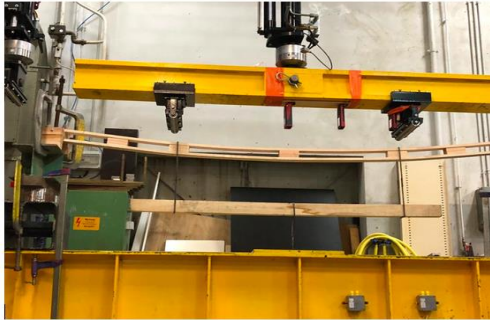
FIGURE 2. Beam without connection in test.
