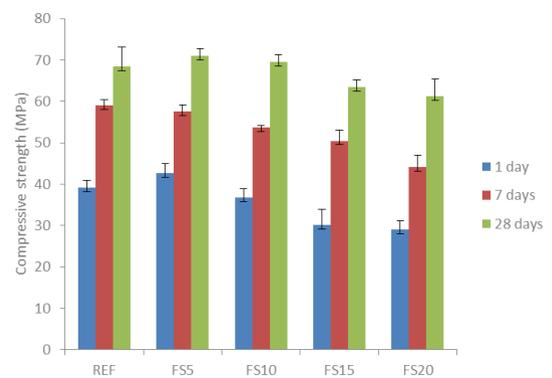
**FIGURE 5.** Compressive strength of mortars
