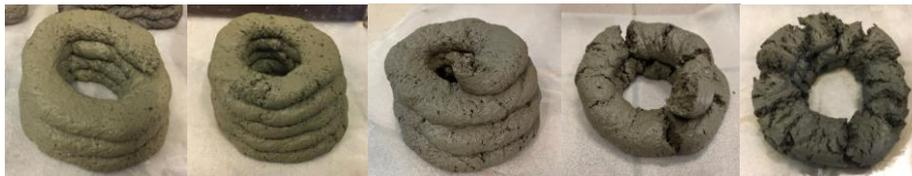
**FIGURE 1.** Printed mixes with the manual gun device (REF – FS5 – FS10 – FS15 –FS20)
