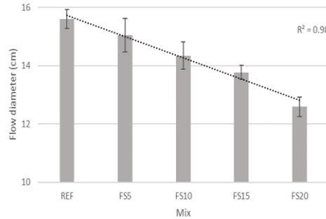
**FIGURE 3.** Variation of flow diameter with the addition of flash-calcined sediment
