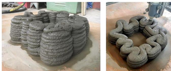
**FIGURE 2.** FS10 mix printed with a gantry Mini Printer
