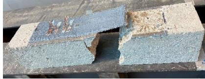
Figure 7. Debonding of the composite and concrete
