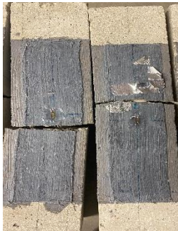
Figure 6. Failure of flax composite
