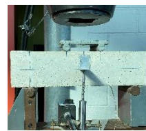
Figure 4. Four-point bending test
