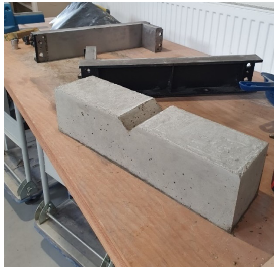
FIGURE 1. SENTMI sample featuring a notch in the middle, after removing the formwork.
