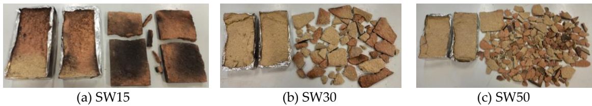
Figure 3. Thermal instable samples (a) SW15 (b) SW30 (c) SW50
