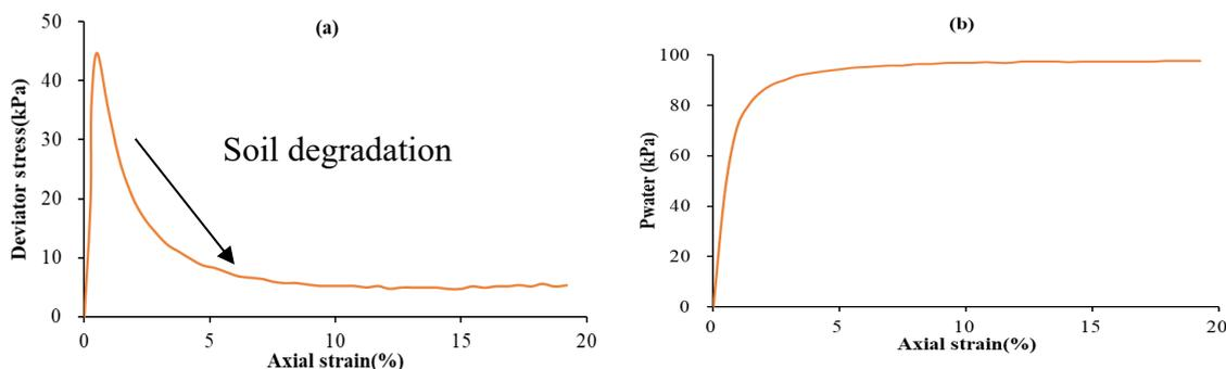
**FIGURE 4. Experimental relation curve between measured excess pore water pressure, deviatoric stress with axial strain of fully saturated Hostun sand RF [11]
