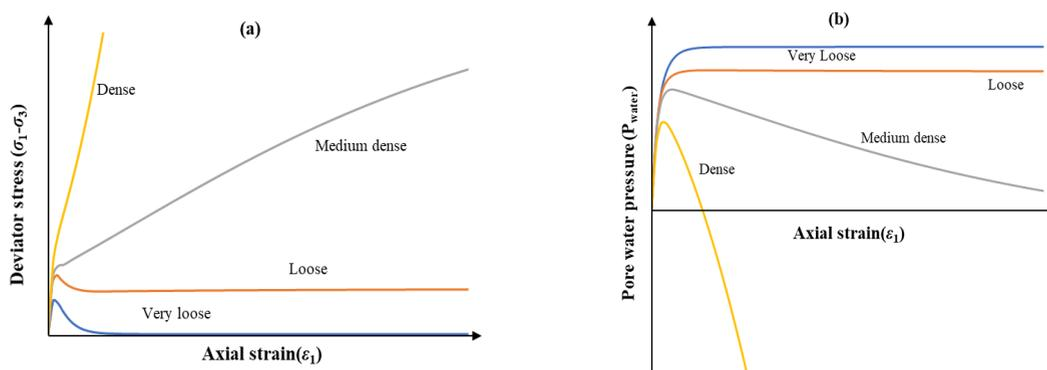
**FIGURE 3. Triaxial undrained test of saturated sand [21]:**
