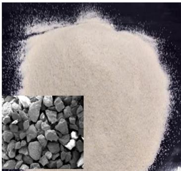
**FIGURE 1.** Hostun sand RF under the microscope [6]
