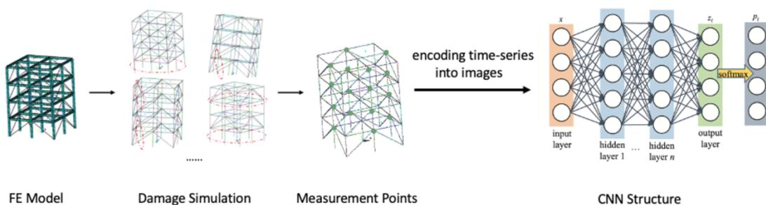
**FIGURE 2.** General pipeline of structural damage detection
