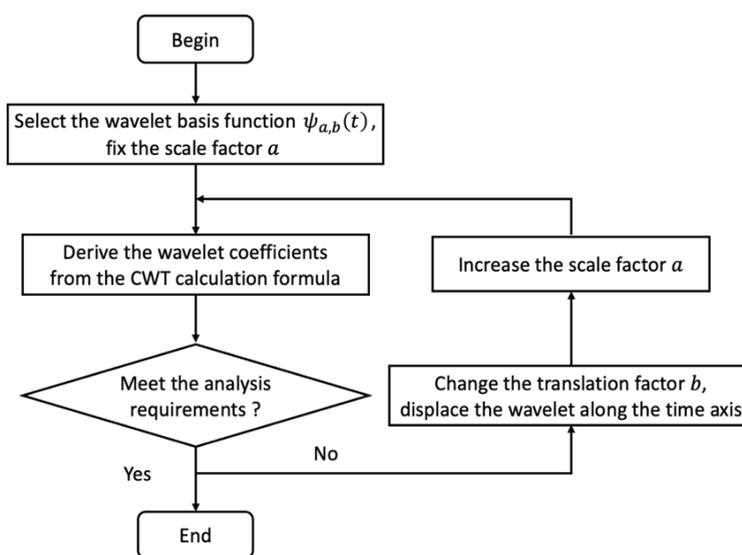
**FIGURE 4.** Numerical Basic flow of Wavelet Transform
