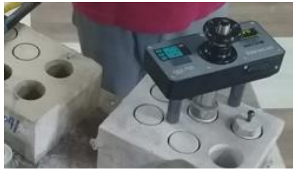
FIGURE 2: test d'arrachement PULL OFF
