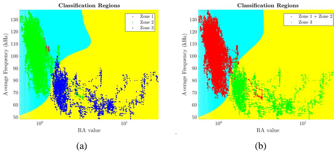
**FIGURE 6. SVM classification using Gauss kernel: (a) three labels, (b) two labels (sample 2)**
