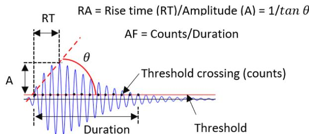
**FIGURE 1.** Schematic representation of an AE signal and definition of some important AE parameters
