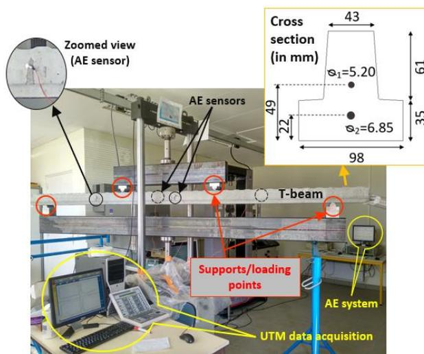
**FIGURE 2. Experimental set-up: UTM, AE-setup, and sample beam ( $\varnothing_1, \varnothing_2$  -are diameters of longitudinal steel).**
