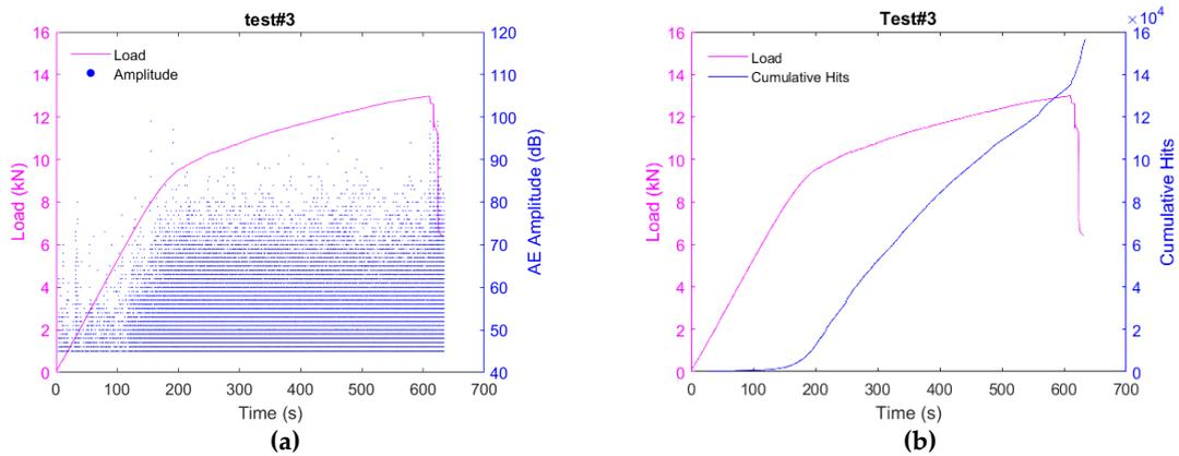
**FIGURE 4.** (a) Variation of load and AE amplitude with time, (b) variation in cumulative AE hits with time (sample 3)
