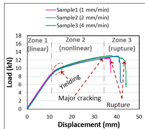
**FIGURE 3. Load-displacement curves of the three samples obtained from the test**
