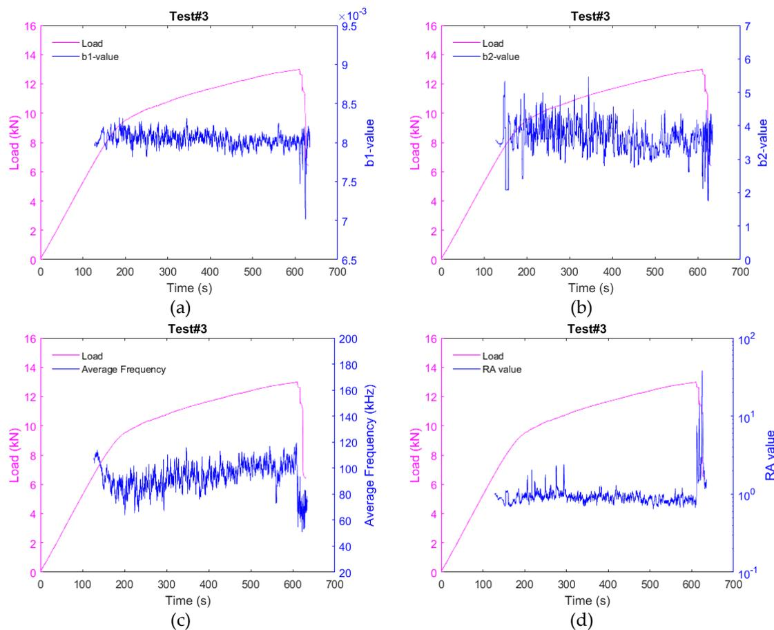
**FIGURE 5.** Evolution of (a) b1-value, (b) b2-value, (c) Average frequency, and (d) RA-value (sample 3)
