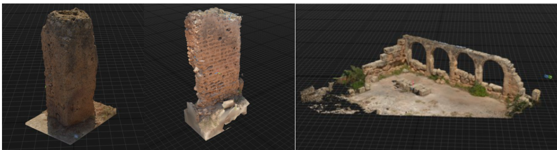
FIGURE 3. The reconstructed raw model from RealityCapture
