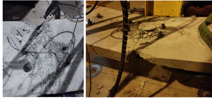
FIGURE 6. Crushing of the intermediate concrete block during phase (e)
