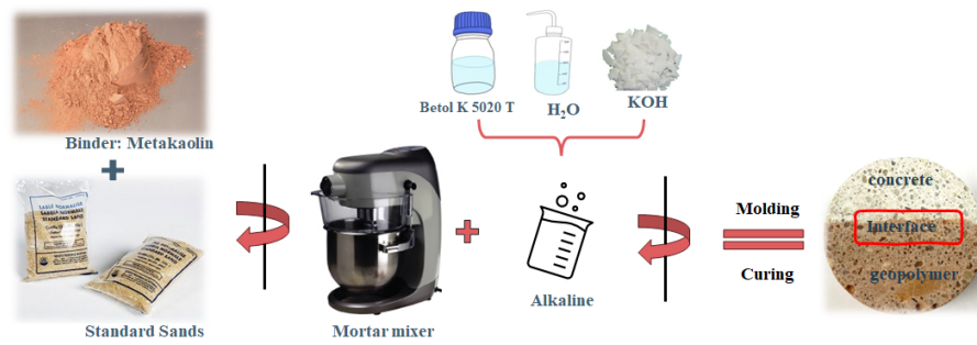
FIGURE 1. Geopolymer Mortar Preparation Flowchart
