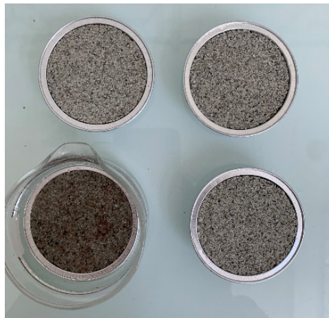
FIGURE 2. Specimens for cone penetration tests
