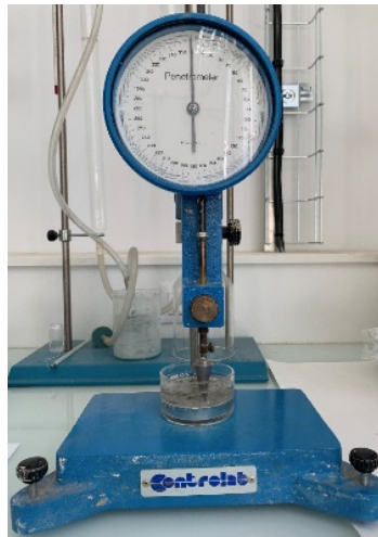
FIGURE 3. Cone Penetration Test
