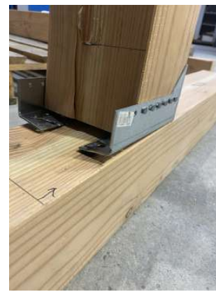
(c) TC: Yielding of the metal clamp and pull-out of the screws
