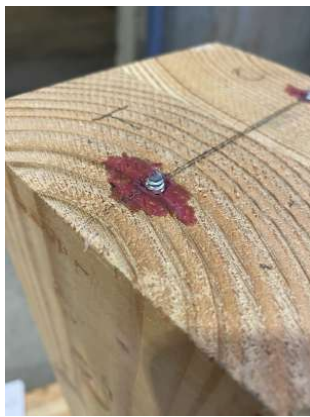
(a) NG-2: ductile failure
