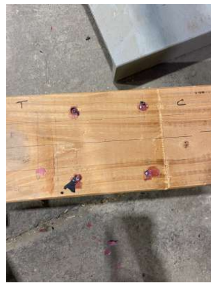
(b) NG-4: ductile failure
