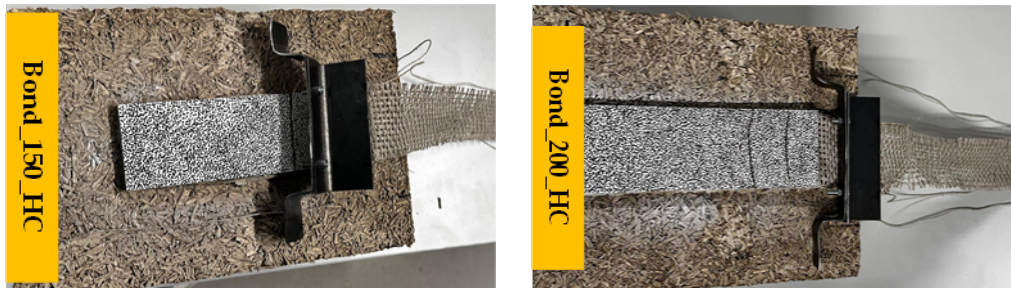
Figure 14. Mode de rupture
