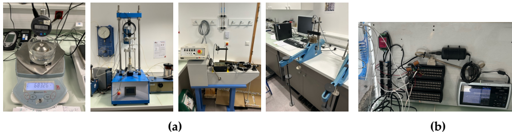
FIGURE 4. Geotechnical tests and data acquisition framework: a) tests to determine the soil's mechanical properties; b) GL800 Graphtec data acquisition unit
