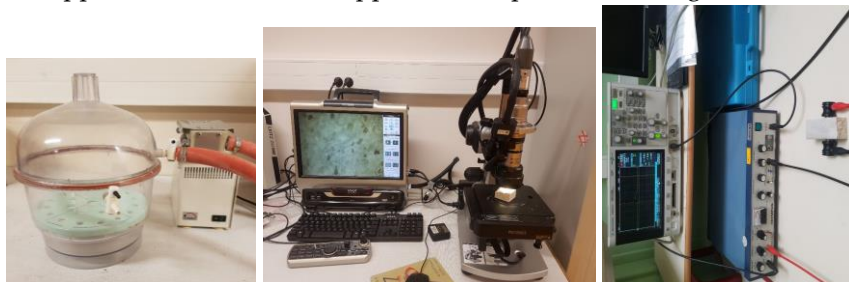
FIGURE 2. Porosity system, Microscope and Ultrasonic apparatus
