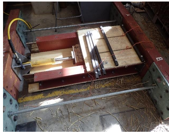
Fig. 3: Set-up for compacting prototype bales.
