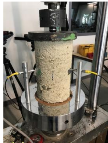
Fig. 1: Simple compressive strength Test.
