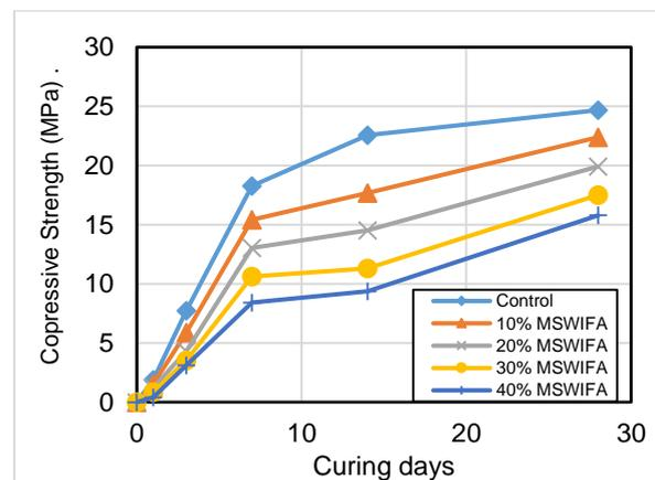
Fig 2 Effect of curing duration on compressive strength.
