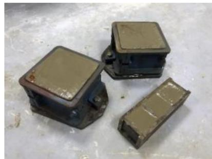
Fig. 1. Mortar specimens.
