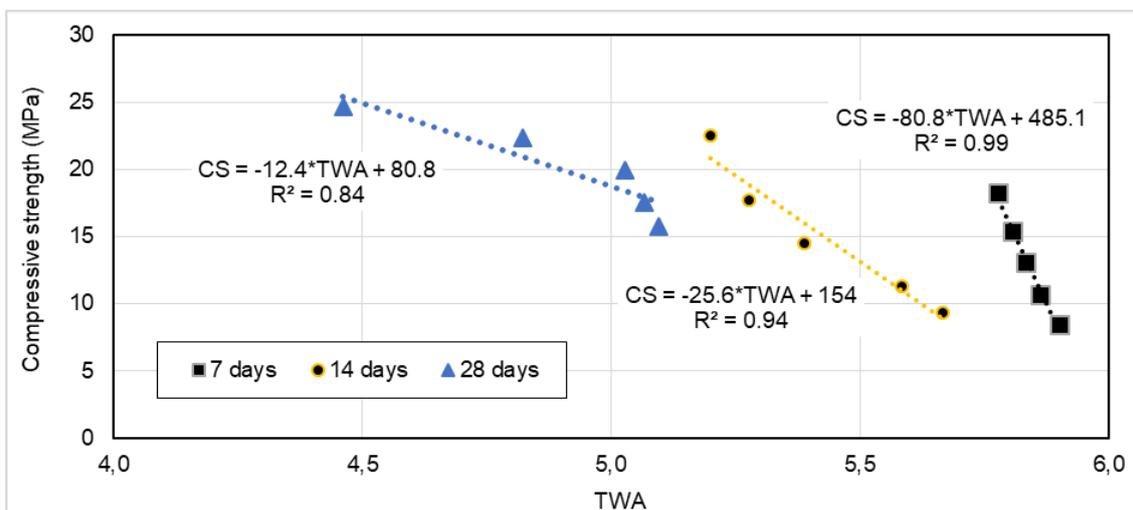
Fig. 10 Correlation between compressive strength and TWA.
