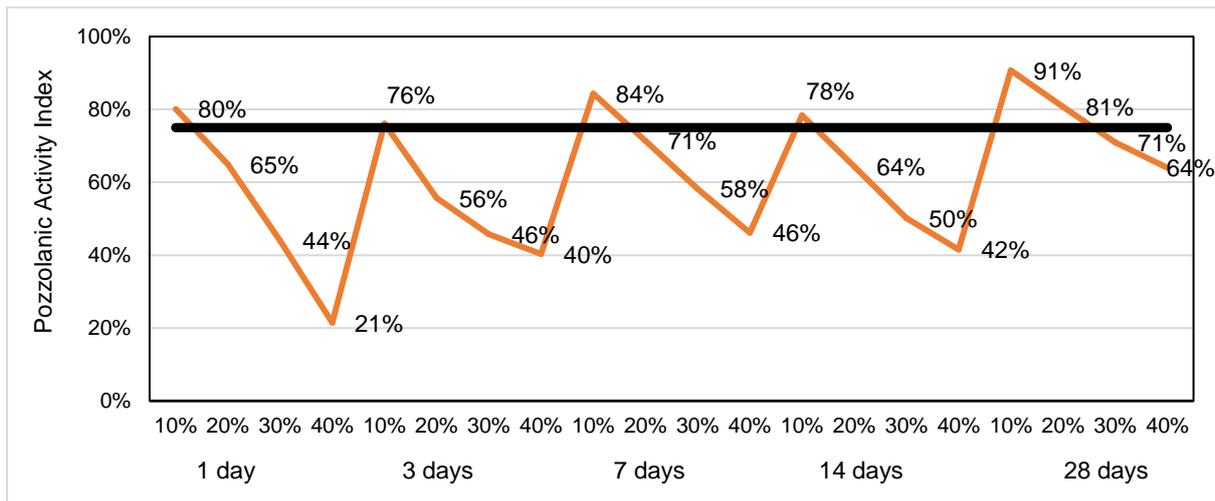
Fig. 5. Pozzolanic activity index for the various mixes.
