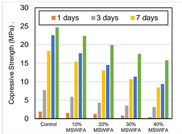
Fig. 3 Effect of MSWI-BA on compressive strength.
