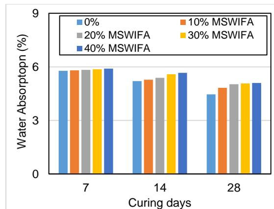
Fig. 8 Effect of curing durations on TWA.
