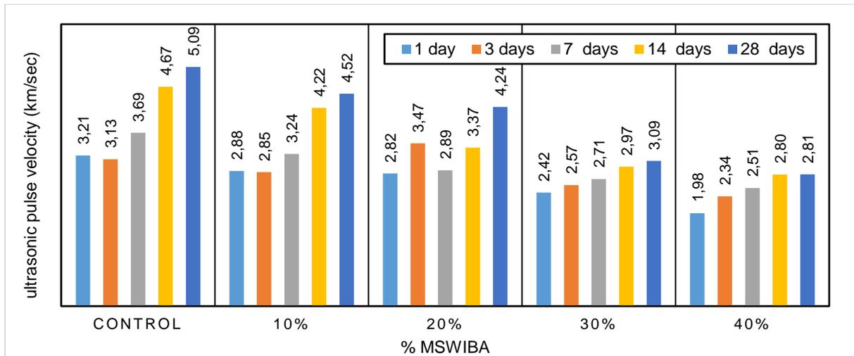
Fig. 6 UPV for the various mortar mixes.
