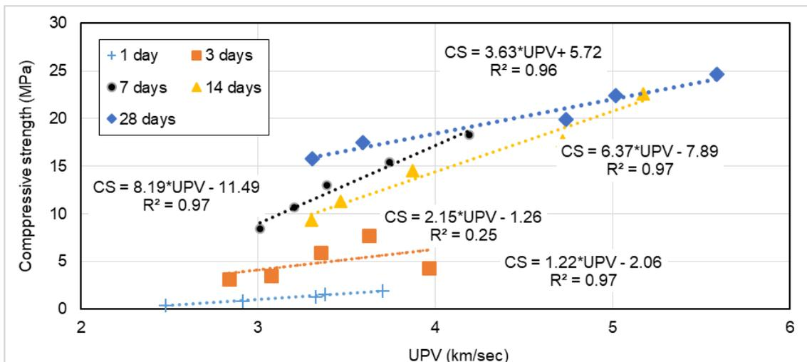
Fig. 9 Correlation between compressive strength and UPV.
