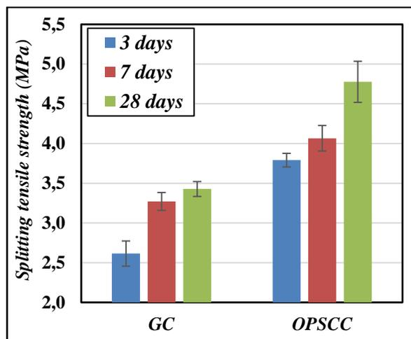
Fig. 34: Splitting tensile strength evolution of geopolymer and OPC concretes.
