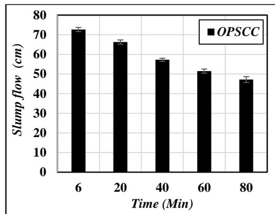
Fig. 31: Slum flow evolution of OPSCC as function of time.
