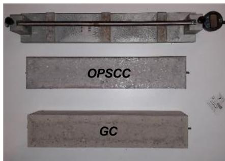
Fig. 30 : Drying shrinkage measurement apparatus and concrete beams.
