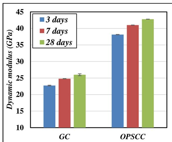
Fig. 35: Dynamic modulus evolution of geopolymer and OPC concretes.
