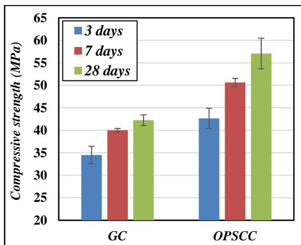
Fig. 33: Compressive strength evolution of geopolymer and OPC concretes.
