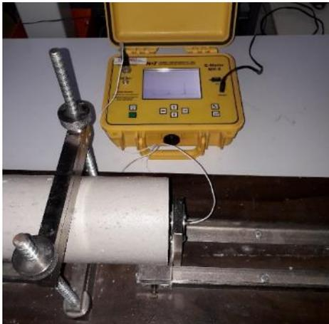
Fig. 29 : Dynamic modulus of elasticity test using E-Meter K II instrument.
