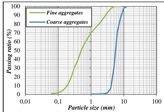
Fig. 28: Grading curves of fine and coarse aggregates.
