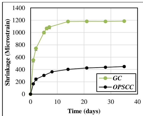
Fig. 37: Dry shrinkage of OPSCC and GC stored at 20°C and 50% RH.
