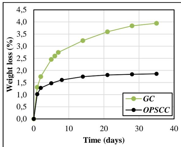
Fig. 36: Weight loss percentage of OPSCC and GC stored at 20°C and 50% RH.
