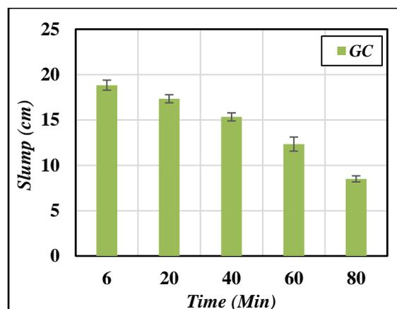
Fig. 32: Slump evolution of geopolymer concrete (GC) as function of time.
