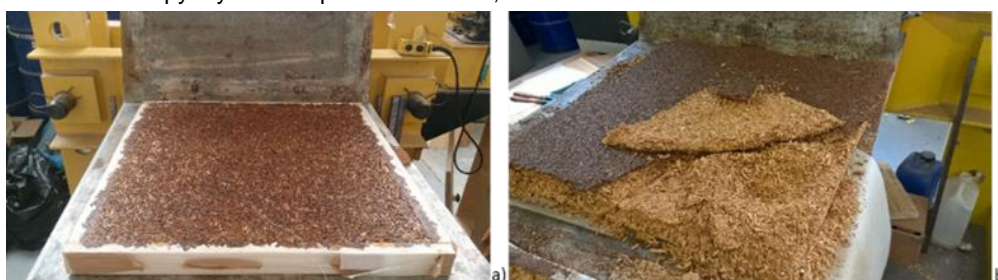
Fig. 11 : Effect of fire retardant treatment on panel aspect (a. untreated, b. Sulfuric acid treated)
